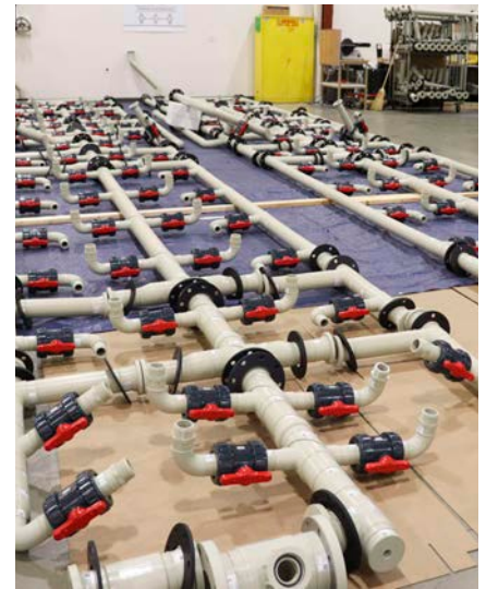
Example of a ultrafiltration skid that will be installed in a trailer
