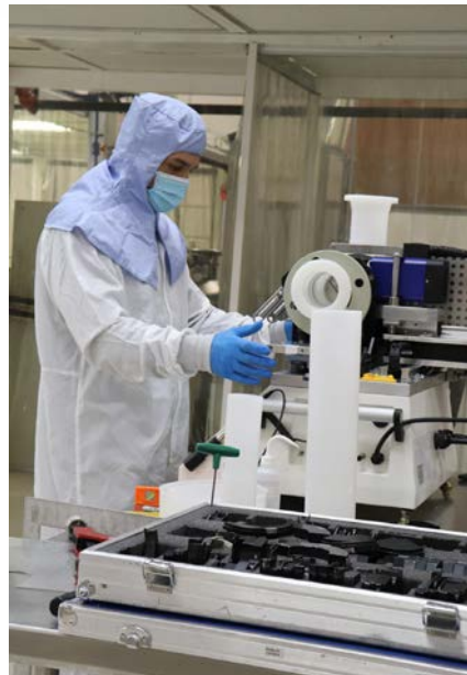
Asahi/America's ultra high purity piping spools fabricated in our class 1000 cleanroom
