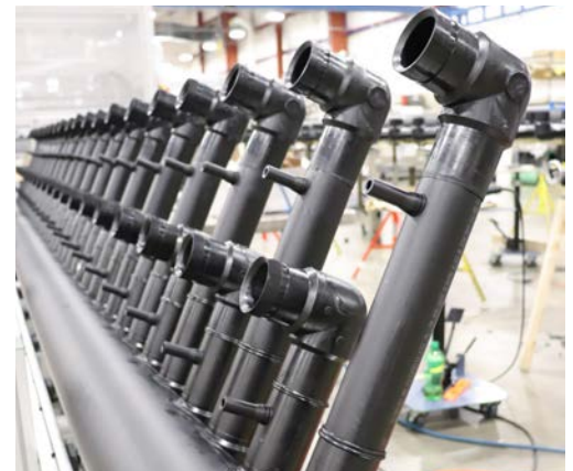
Example of a ultrafiltration skid that will be installed in a trailer
