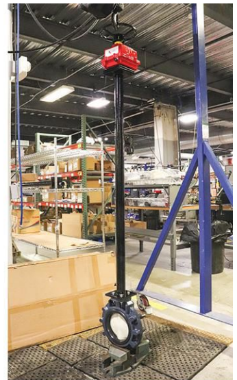
IMAGE 1: A butterfly valve with an added chain wheel option to the gear operator (left) and powder-coated stem extension with an electric actuator (right). (Images courtesy of Asahi/America, Inc.)
